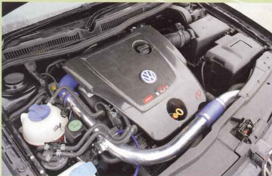
Above: boasting a bigger charger, larger intercooler and ECU remap, the 1.9 turbo-diesel lump provides over 310lb.ft of torque
